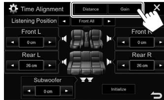
**[Distance]** Adjusts the Digital Time Alignment (DTA) value.
