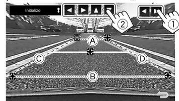
Make sure that (A) and (B) are horizontally parallel, and that (C) and (D) are the same length.
